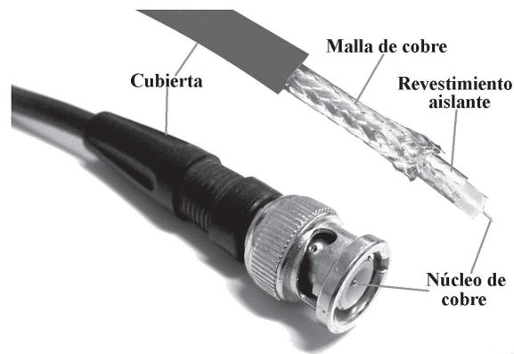
Figura 1.30. Cable coaxial
